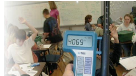
Carbon dioxide in classroom: adult critical thinking declines at 1,000 ppm CO2
