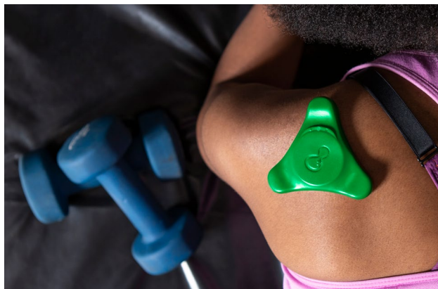
The ADAMM wearable device measures health parameters for asthma and connects with the Nightingale platform.
